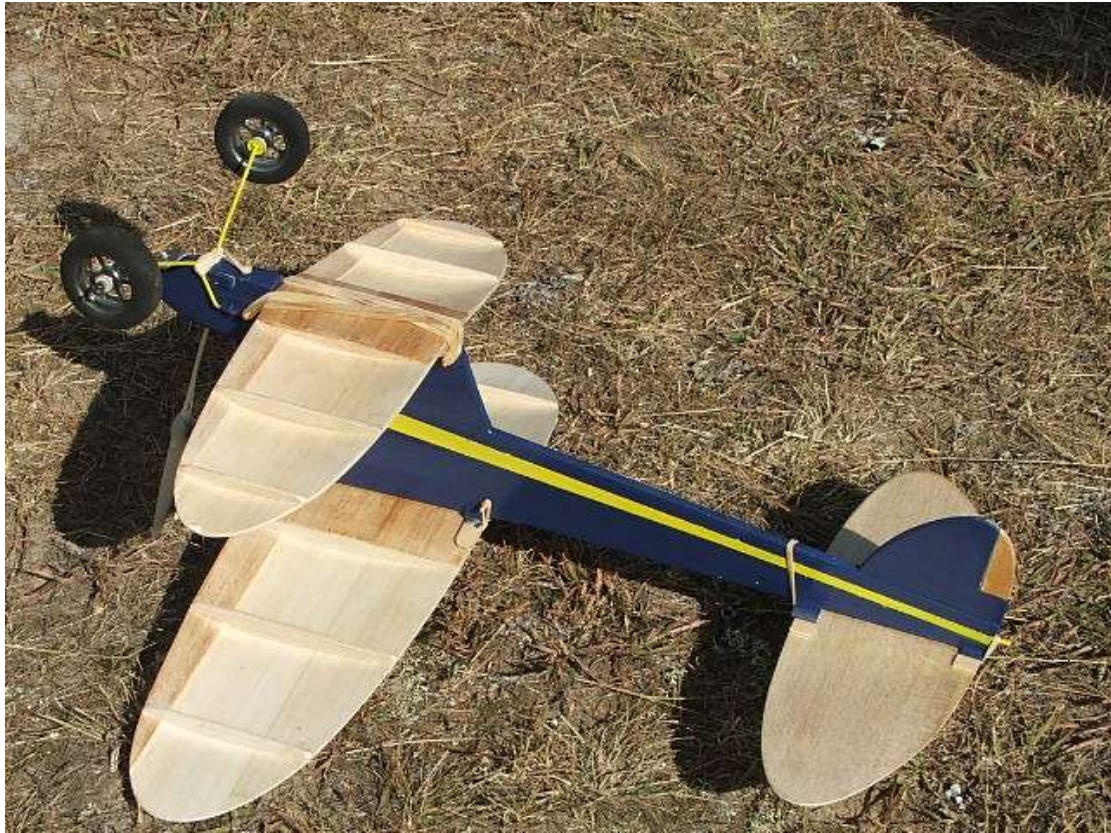
Underside of Brian's Mimi showing rib placement and reinforced LE.
